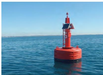
*The new buoy being trialled has better stabilisation, safer storage of electronics and batteries, advanced communication and monitoring technology for maintenance purposes and tracking and rubber mooring, which keeps the buoy in correct position.*
