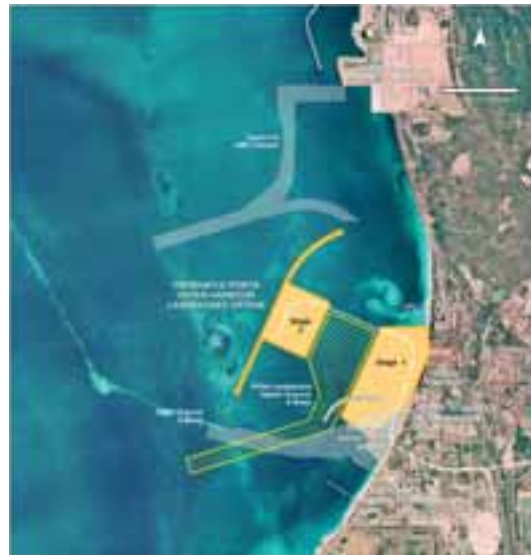
The second option is a partially land-backed facility located just south of Alcoa that would include reclamation of the foreshore and an island component with a freight link via Anketell Road.
